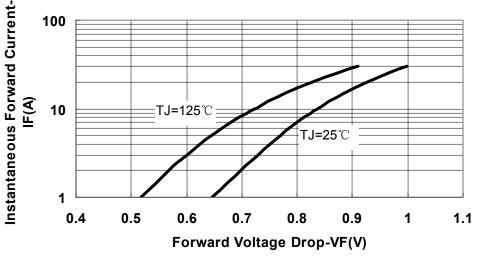
Fig.3-Typical Instantaneous Forward Voltage Characteristics
